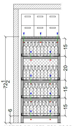
17, 24, 32.5" deep bottle shelf starts at 6" AFF. Shelf heights are fully customizable. Hot dipped galvanized finish standard or powder coated to specific colors on any and all pieces. Assemble with included Grade 5 hardware.
